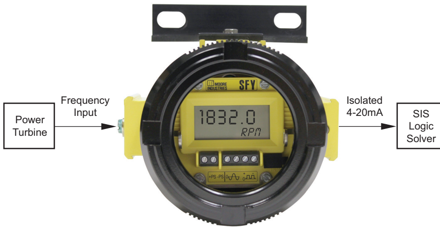
Figure 7.1. Turbine Over Speed Protection System
